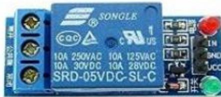
**Gambar 3.18 Relay 5V 1 Channel**
