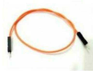
**Gambar 3.21 Kabel jumper male to male**
