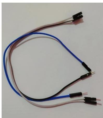
**Gambar 3.20 Kabel Jumper**
