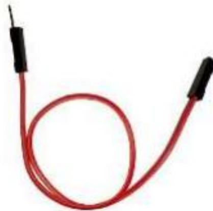
**Gambar 3.22 Kabel jumper male to female**
